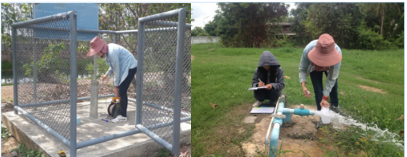
Figure 1 – Protection of the observation well (left) and the process of reading the measurements (right)
