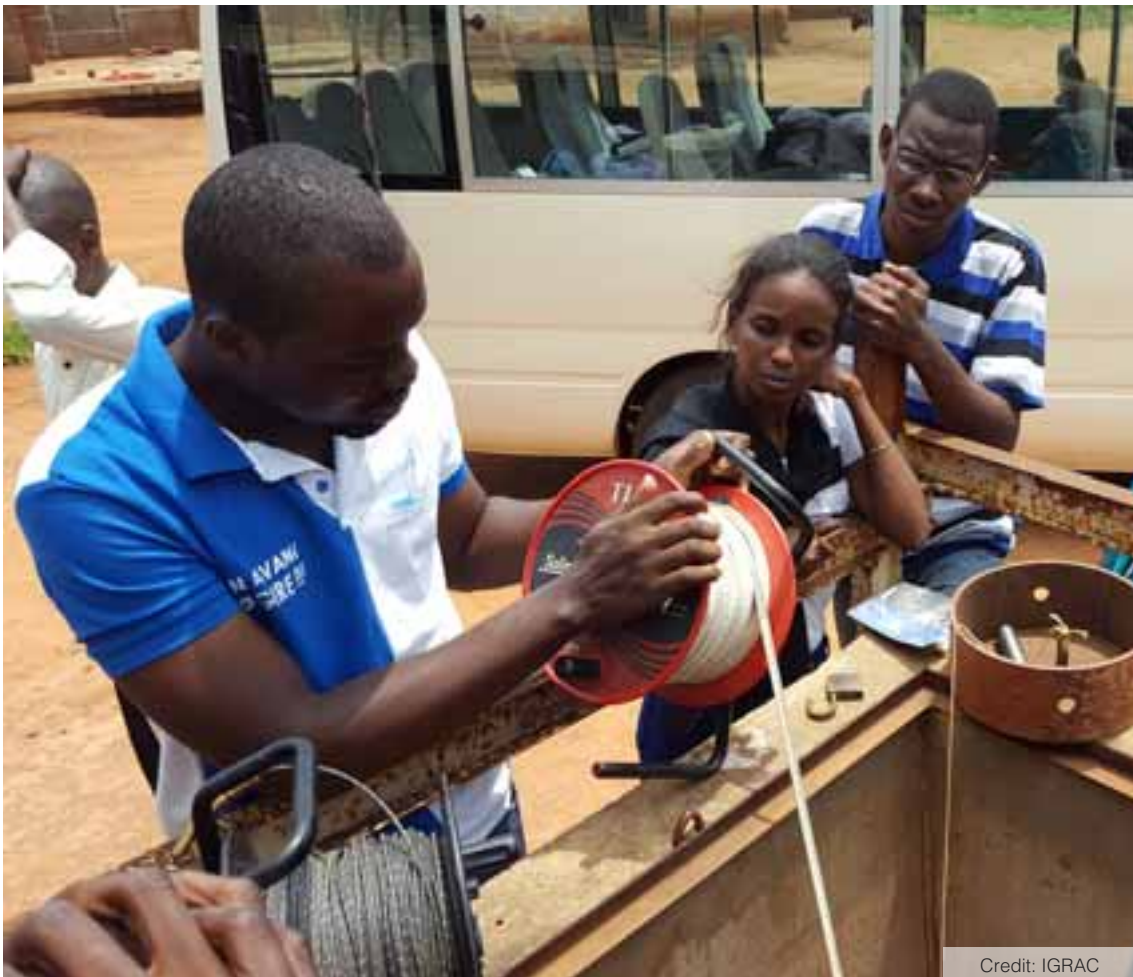
Measuring of water levels is part of groundwater monitoring
