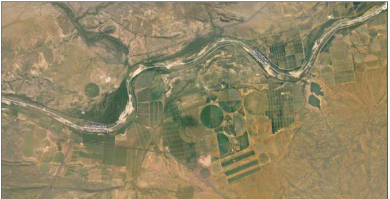
Figure 2: Detail showing the irrigated areas with Centre Pivots (2000 ha) and rectangular field (4500 ha) layouts. Rectangular fields are largely Citrus, and centre pivots are for cotton. Limpopo river runs west to east through the middle of the image.
